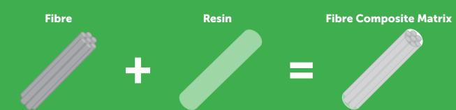
Provides strength and stiffness (glass, carbon, aramid, basalt, natural fibres)
